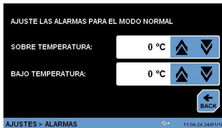
Fig. 8.5 Setting alarm margins
